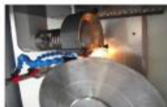
HSS circular saw grinding
